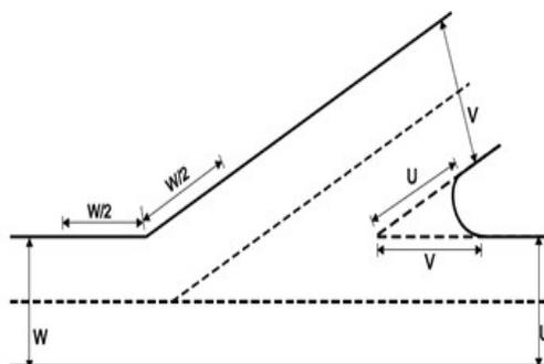
**Fig.3B** - Rounding off at junctions at acute / obtuse intersections.
